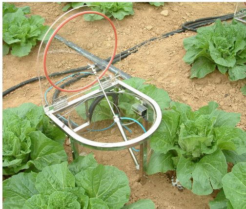
Fig. 1. Steady-state chamber for collecting N 2 O in soil.
