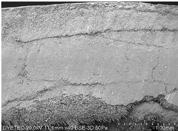
Figure 6. SEM image of the cross-section of 3D braided composite tube.
