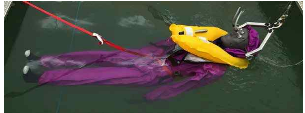
Fig. 5 Test 3 - standard clothing + full body suit with inflatable PFD
