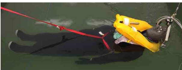
Fig. 3 Test 1 - standard Clothing + inflatable PFD only
