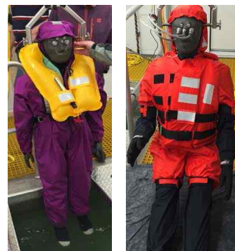
Fig. 7 Lifejacket tested: inflatable with full-body suit (left); foam with short sleeves and legs (right)
