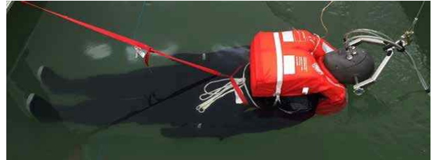
Fig. 4 Test 2 - standard clothing + SOLAS-approved lifejacket
