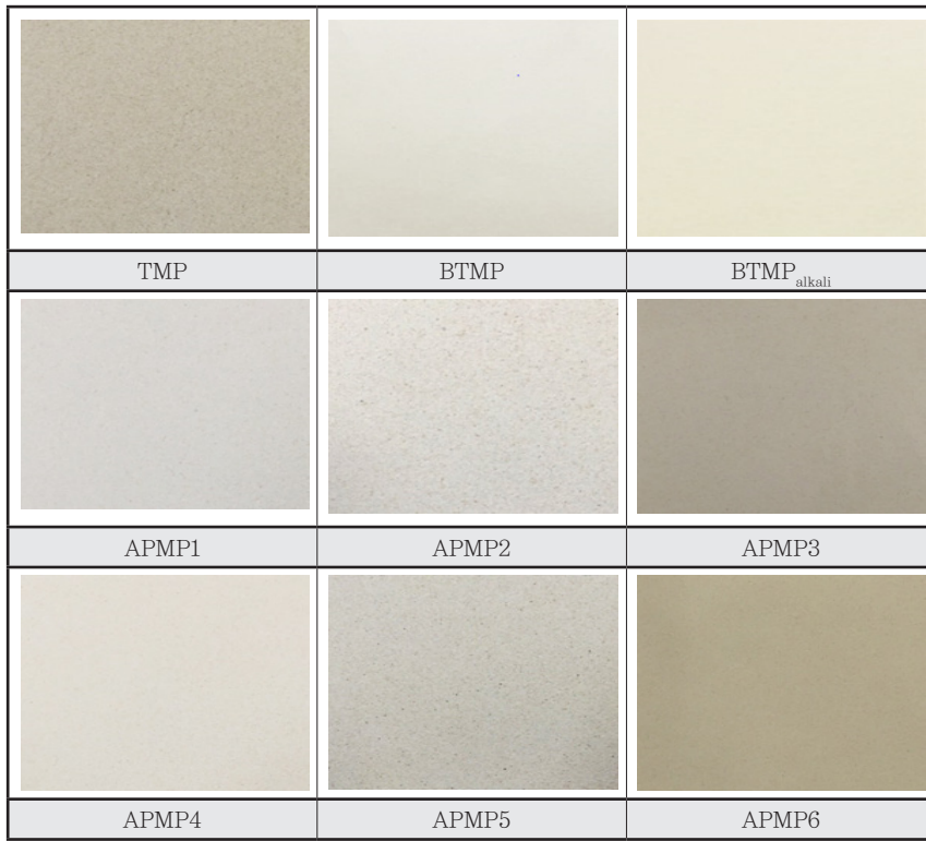
Fig. 8. Color comparison of TMP and APMP according to varied mixing ratios of liquors.
