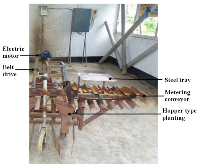
Figure 3. Laboratory set-up for the evaluation of the performance of the planting device.
