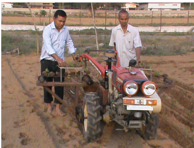
Figure 7. Operation of 2-row hand-tractor-powered vegetable transplanter with hopper-type planting device.
