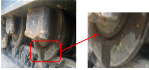
Fig. 2 External leak of track roller
