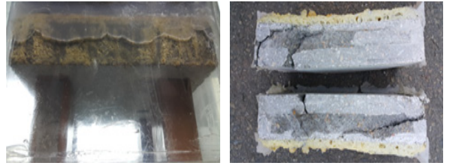
(a) rear (b) section Fig. 23 Test specimen indirectly exposed to water by covering with soil
