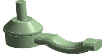
[Fig. 3] C type tie rod end model
