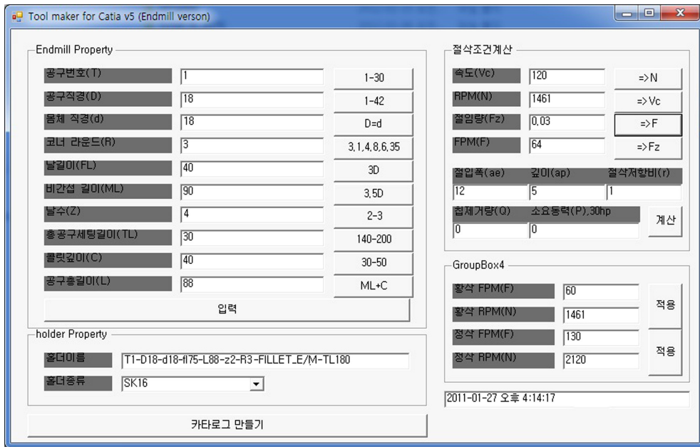
Fig. 4 Maximum spindle speed and feed rate of vertical machining center calculated by CATIA V5 tool maker
