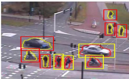
[Fig. 1] Tracking of The Car Object
