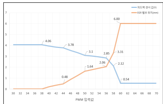
Fig. 20. Feedback sensor value and EGR valve position according to PWM input value
