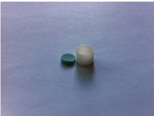
Figure 1. Sample and cup holder for TG test.
