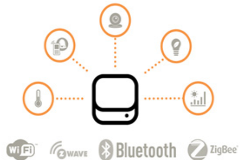
Fig. 5 Supporting Various Network Protocols in out IoT Gateway
