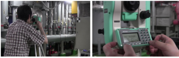
Figure 5. Total station based distance measurement for checking scan quality
