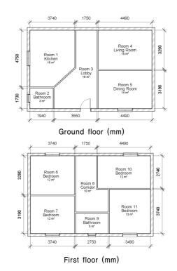
Figure 2. Floor plan for a typical detached house
