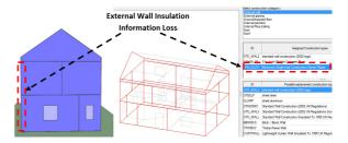
Figure 4, Construction information loss in IES VE/IMPACT
