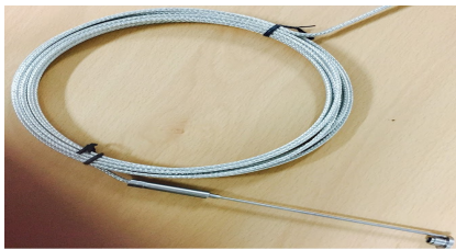
[Fig. 5] Temperature Sensor
