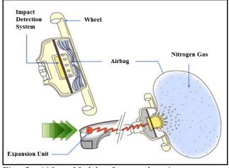
Fig. 3. Airbag Module: Impact detection system + Expansion unit + Airbag.
