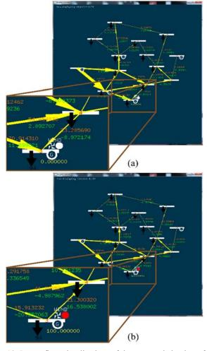
Fig. 10. Power-flow visualizations of the proposed simulator for IEEE 14 bus system with wind power generator at time slot. (a) At t = 4, (b) At t = 11.
