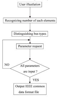
Fig.4. Flowchart of generations of IEEE common data format files.
