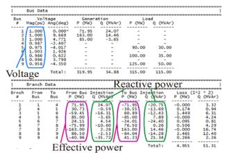
Fig. 9. Power flow calculation results from MATPOWER.
