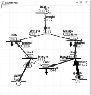
Fig.7. System diagram of IEEE 9-bus system drawn by authors.
