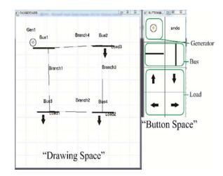
Fig. 5. Drawing window of the proposed simulator.
