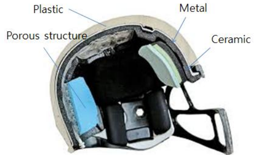
Fig. 1 Typical helmet cross section structure
