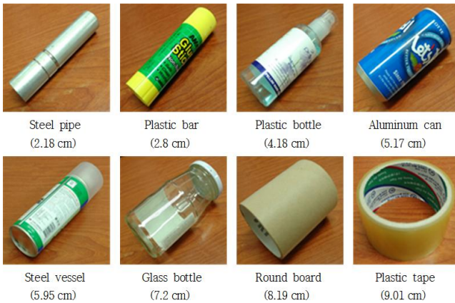
Fig. 8 Cylindrical objects used in the experiments. The diameters of mundane objects varied from 2.18 cm to 9.01 cm.
