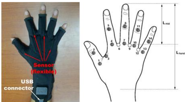
Fig. 5 5DT 14-Ultra, Fifth Dimension Technology Co. (left) and Placement of 14 sensors in the data glove (right)
