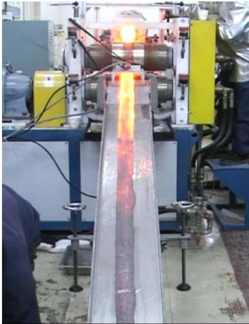
Fig. 3. Strip casting of bulk amorphous composite alloy (RIBA 503 alloy specimen).
