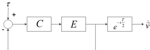
Fig. 5. Time delay separating system of Smith predictor
