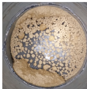
Fig. 2. Clumped wood particles at the bottom of the drying tower.
