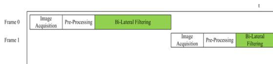
Fig. 8 Using universal GPU parallel programming timing chart
