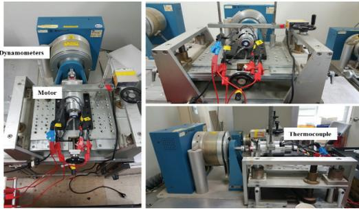
Fig. 2 Experiment equipment for motor load test
