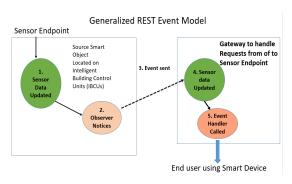
Fig. 2 Generalized REST Event Model to be implemented in the proposed IoT Gateway
