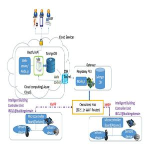
Fig. 1 A prototype architecture for Intelligent Buildings (energy metering, home automation, wireless monitoring) related IoT environment
