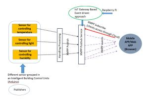
Fig. 3 Design Publish-Subscriber service for collecting and broadcasting new sensor data from IBCUs
