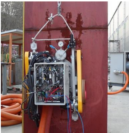
Fig. 2 Photograph of the hull cleaning robot in operation
