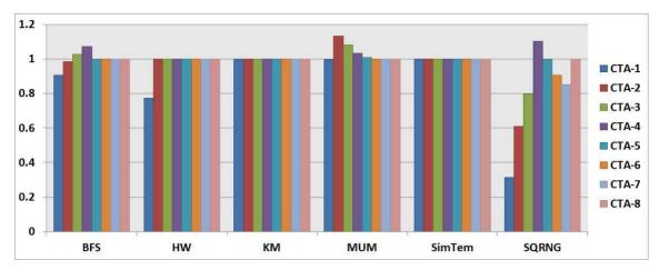
Fig. 3. GPU performance according to number of CTAs assigned to the SM
