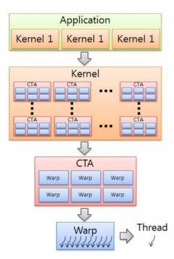
Fig. 2. GPU programming architecture (CUDA)
