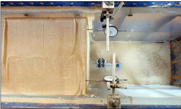
Fig. 7. Top view of dial gauge installation
