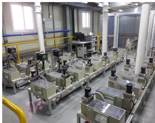
Photo 1. Mixer-settler for scale up test.
