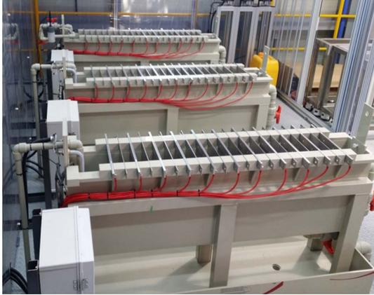
Photo 2. Electro-winning cell for scale up test.
