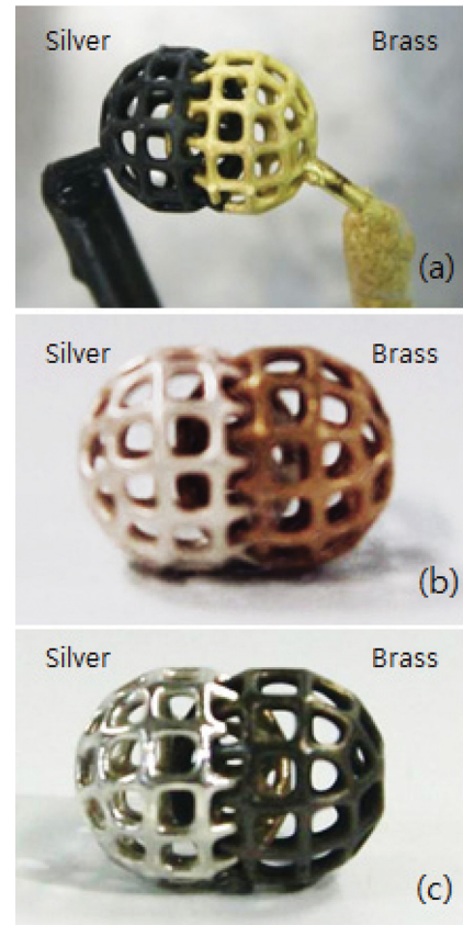
Fig. 3. Dissimilar metals results using 3D printing. (a) Decomposition (b) finishing (c) polishing and metal surface treatment (5NaClO 2 : 1NaOH).
