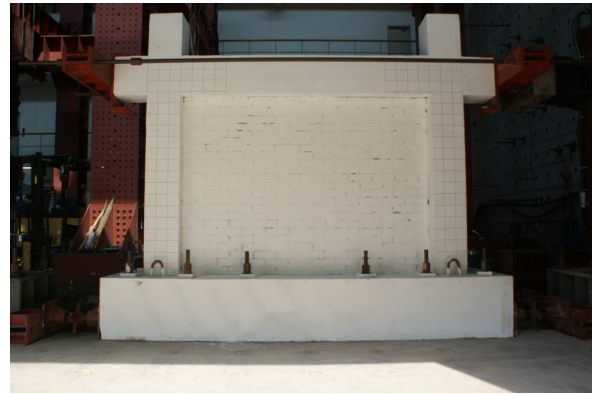
Fig. 1 Masonry infilled frame specimen
