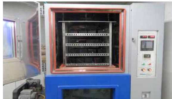
Fig. 5. Photo of freeze-thaw test chamber.
