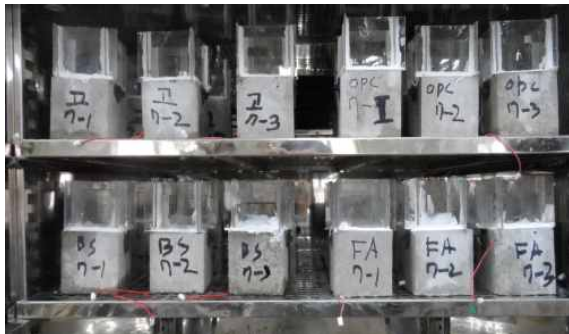
Fig. 8. Photo of ponding freeze-thaw test chamber.
