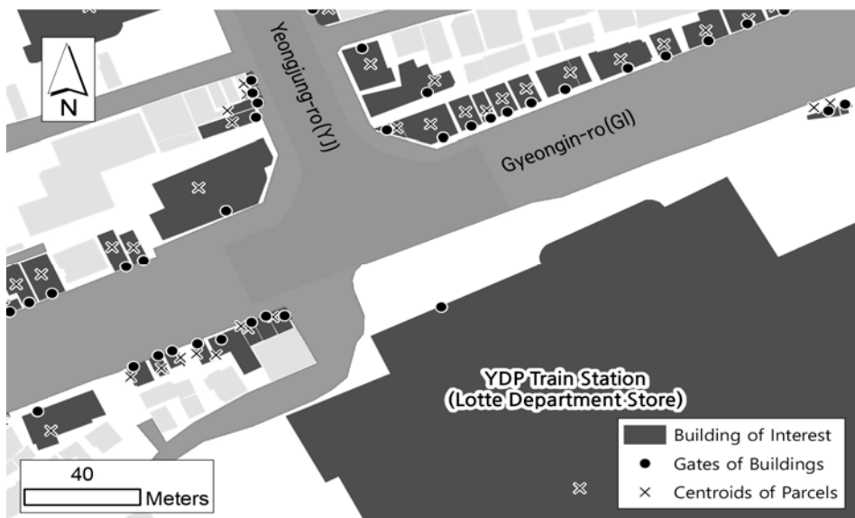
Figure 4. Differences in Address Coordinates between Gate of Building (Road-based) and Centroids of Parcels(Parcel-based)
