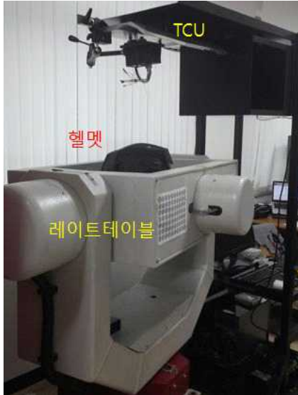
Fig. 8. Accuracy test rig for optical pose tracking(using 3-DOF Rate table)
