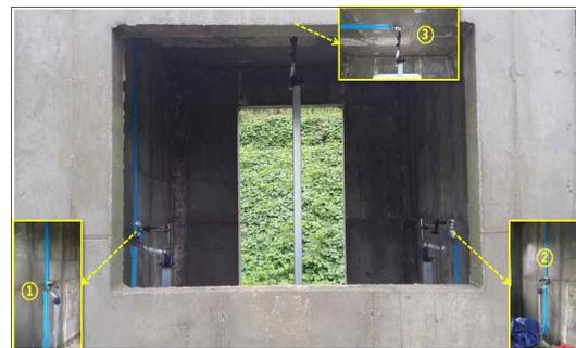
Figure 4. Displacement and acceleration sensors to measure structural deformation
