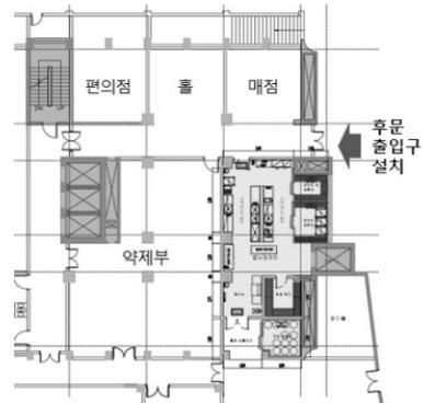
[Figure 16] Remodeling Plan for Catering Department(Basemen 1st Floor)
