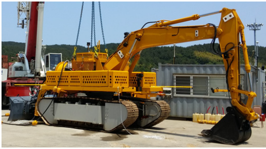
Fig. 1. Underwater equipment for rubble mound leveling
