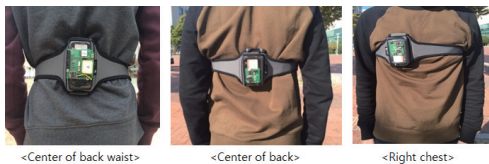
Fig. 11. Mounting positions of PDR module.
