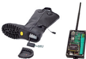
Fig. 3. PDR system for firefighter.
