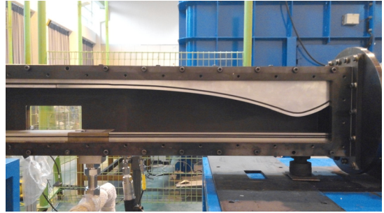
Fig. 2. Experimental Setup for Backward Facing Step
