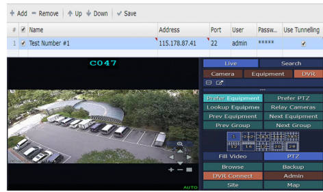
Fig. 5. Remote Access using Tunneling
