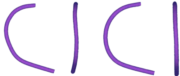
(a) Length of vibrate 0.05mm (b) Length of vibrate 0.1mm Fig. 7 The results of FE-simulation according to the length of vibration
