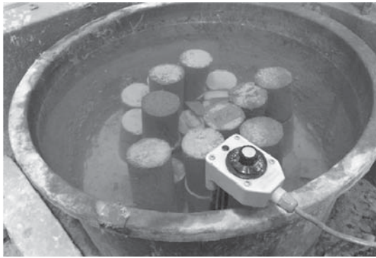
Fig. 3 Curing specimens following ASTM C31.
