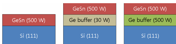
Fig. 1. Schematics of the prepared GeSn films (a) Sample 1: GeSn directly on Si without Ge buffer. GeSn-on-Si samples with Ge buffers prepared at (b) 30-W (Sample 2), (c) 500-W (Sample 3) DC sputtering powers.
