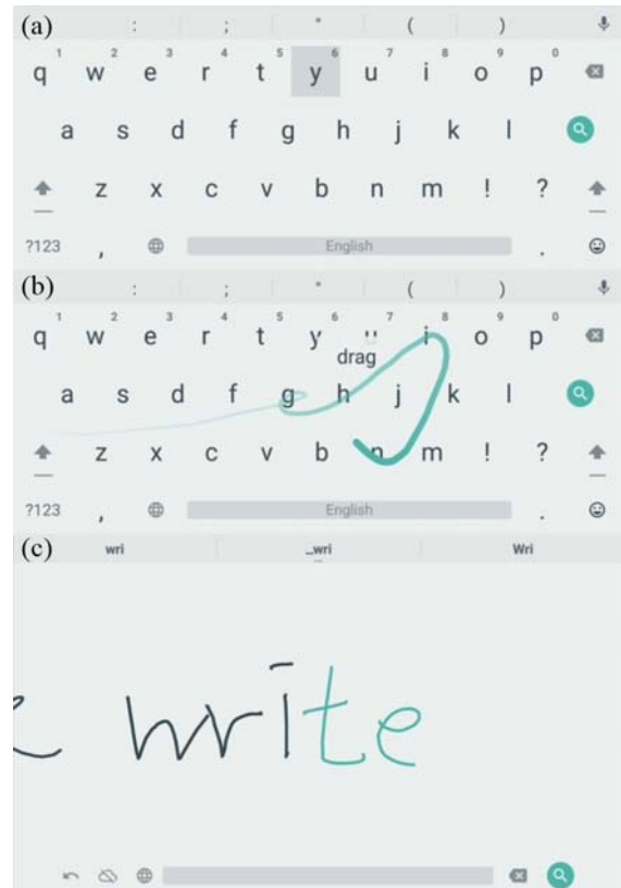
Figure 1. Three Types of Keyboard Applications(each Follows (a) QWERTY, (b) Swype, (c) Gesture)
