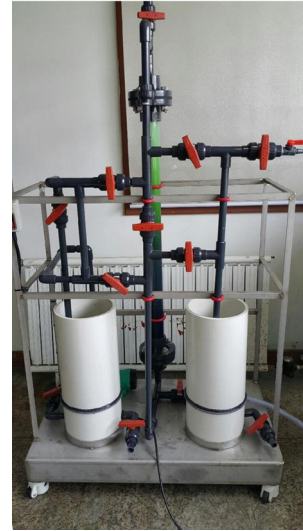
Figure 1. Picture of ion exchange method apparatus.
