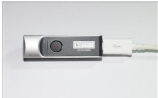
[Fig. 6] Connecting USB IR thermometer (thermometer module)
