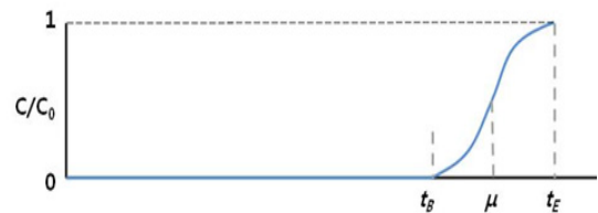
Fig. 4 Typical breakthrough curve of adsorbent
