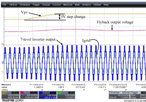
Fig. 19. Experimental results showing the 7-level output voltage balanced during a PV step change.
