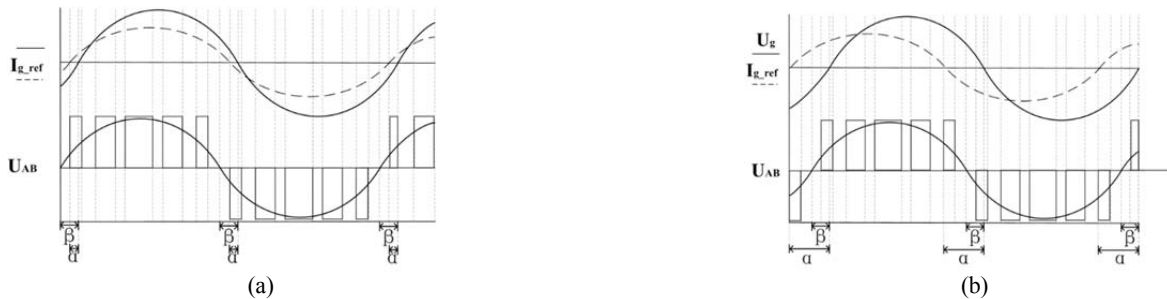
Fig. 10. Waveforms of the hybrid modulation strategy for a leading power factor: (a) \alpha < \beta , (b) \alpha > \beta .
